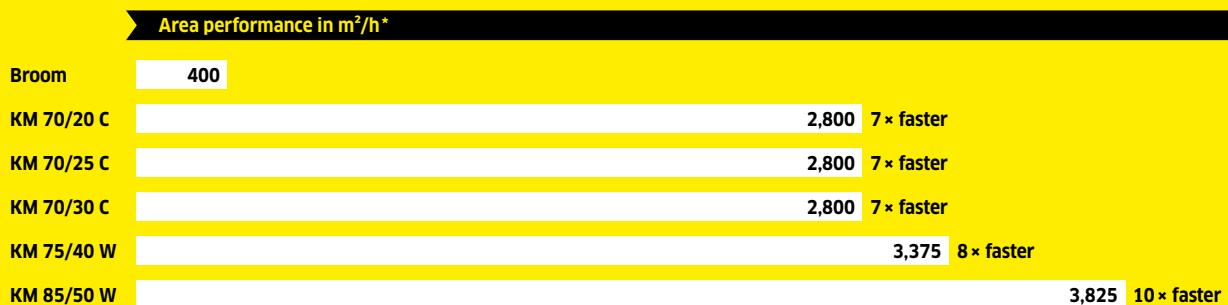
Area performance of a vacuum sweeper compared with employee using a broom.
