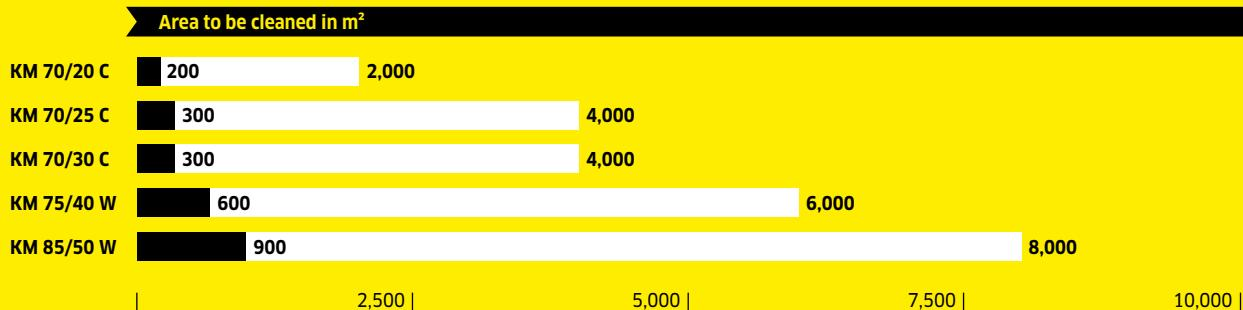
\* Cost-effective range, figures: minimum surface area in m<sup>2</sup> above which using the machine is cost-effective.
